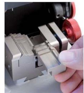
Interchangeable jaws for laser and dimple keys
